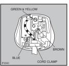
The wire coloured green and yellow must be connected to the terminal marked with the letter «E» or by the earth symbol  $\downarrow$  or coloured green and yellow.
